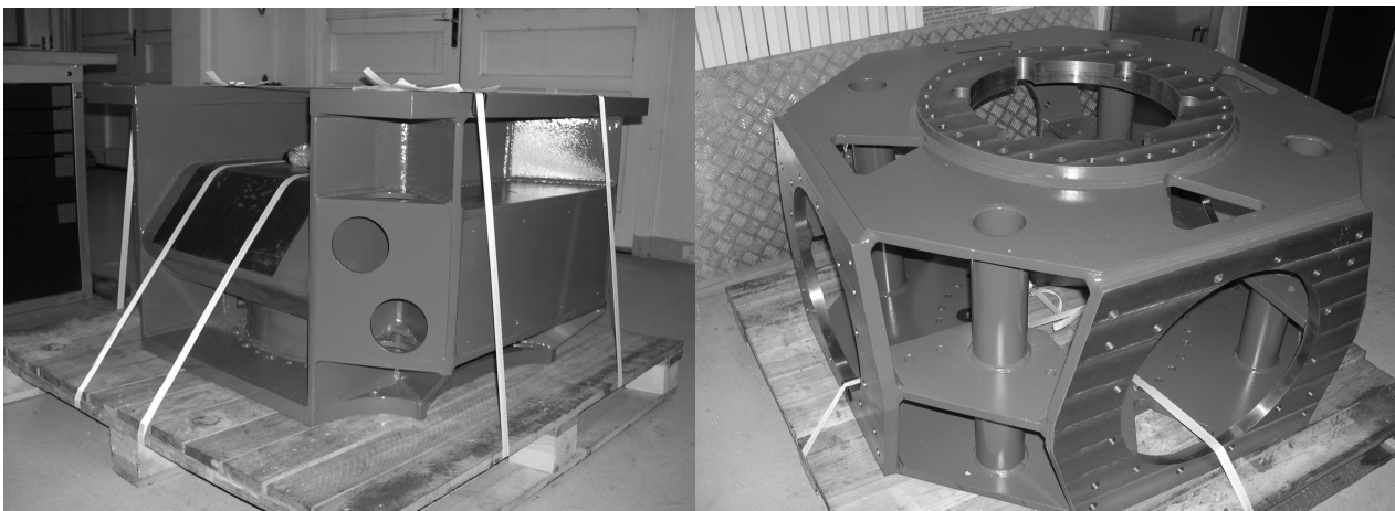
Figure 4: Image of the fork (left) and the bosshead (right) at the Observatory of Paris before their mounting.
