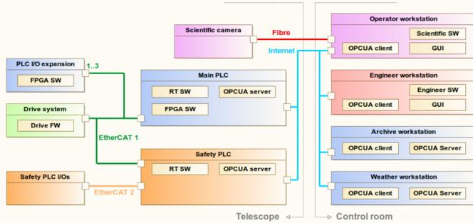
Figure 1: There are only two physical links between the telescope and the control room for communication purposes. A dedicated EtherCAT field-bus is used for safety. The logical connectivity is managed by OPC UA clients and servers. The network devices, such as switches, are not shown. HW stands for hardware, SW for software and FW for firmware.
