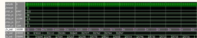
Figure 3: Snapshot of the first iterations of the approximate CORDIC algorithm as simulated by ModelSIM (with 16-bit words in this example). The different entries represent the ports of the component.
