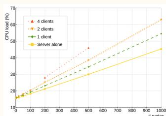
Figure 2: The CPU load of a cRIO9074 while running an OPC UA server. The node values are published by the server and monitored by the clients every second.
