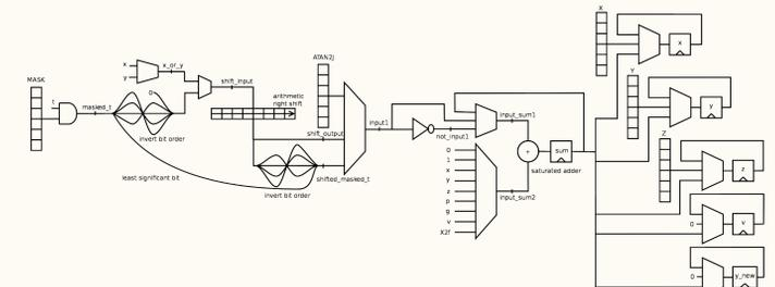
Figure 4: Register-transfer-level (RTL) representation of the XYZ module. This diagram does not show the control logic. Upper case names designate signals read from the read-only memories inside the FPGA (the vertical arrays).
