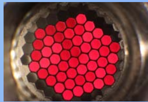
Microlenses array manufactured by AMS
